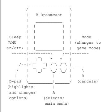
To the left is a drawing of a VMU labelled with all the buttons and controls.
