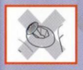
If the Control Stick is held at an angled position (as shown in the picture on the left) when the power is turned ON, this position will be set as neutral. This will cause games using the Control Stick to operate incorrectly.
