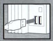
Insert the EyeToy® USB Camera (for PlayStation®2) into either the upper or lower USB connector on the front of the console. The LED
