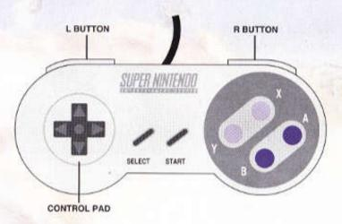
Control Pad ..... Moves characters and controls direction of Trialight.
